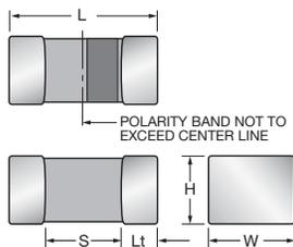
The AVX T4C microchip medical series is designed for use in Implantable - Non-Life support or Non-Implantable - Life support medical applications with space limits. These components are screened using our newly designed Q-Process to effectively remove components that may experience parametric shifts through customer processing or display instability through life testing.
