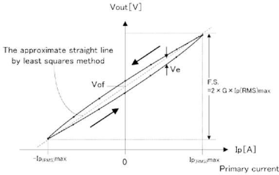
• Sensitivity G [mV/A], Offset voltage Vof [V]
