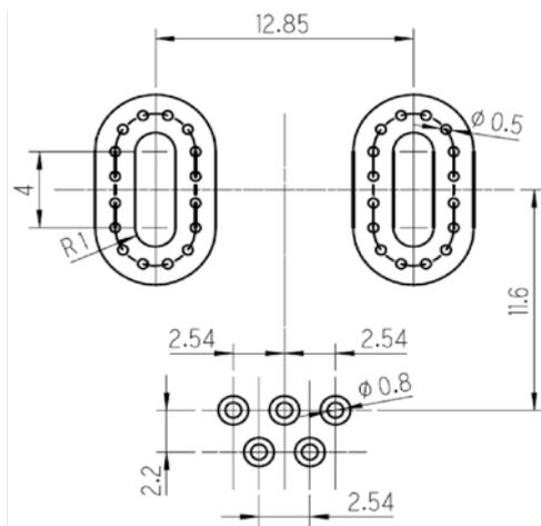
Note) If 2 or more trace layers are used as the current path, please make enough number of through-holes to flow current between the trace layers.
