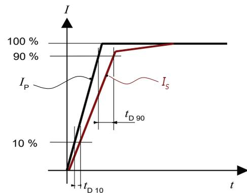
Figure 6:  $t_{D10}$  (delay time @ 10 %) and  $t_{D90}$  (delay time @ 90 %)
