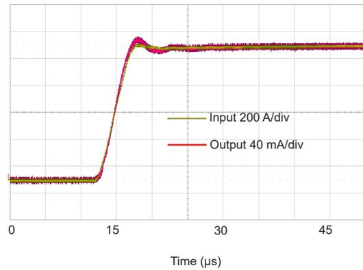
Figure 2: Typical step response (0 to 1 kA, 200 A/μs)
