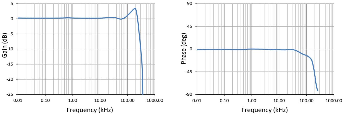
Figure 5: Typical frequency response, small signal bandwidth
