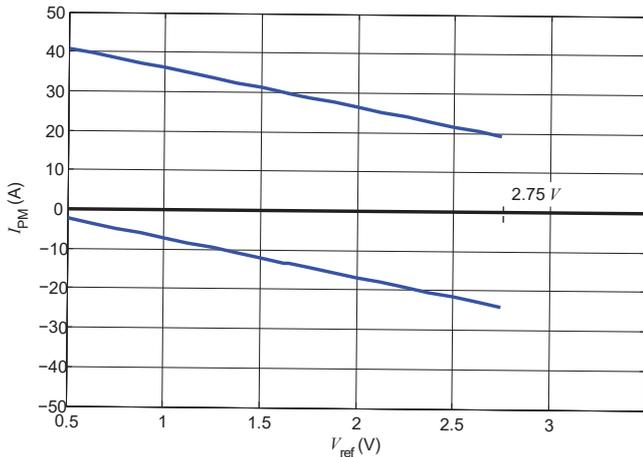
Figure 18: Measuring range versus external  $V_{ref}$
