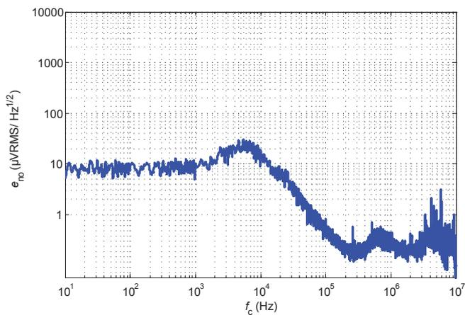
Figure 4: Output noise voltage spectral density
