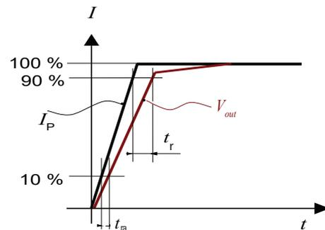
Figure 16: Response time  $t_r$  and reaction time  $t_{ra}$
