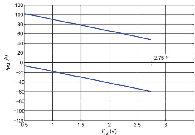
Figure 19: Measuring range versus external  $V_{ref}$
