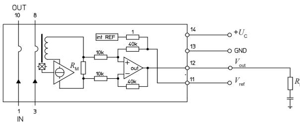
Figure 15: Test connection
