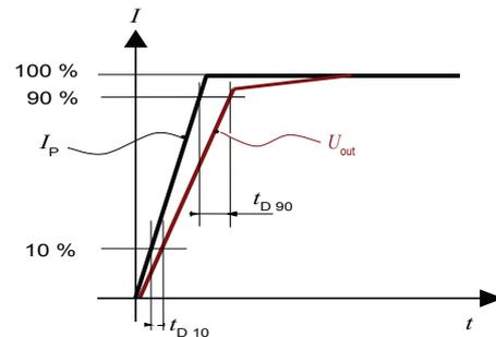
Figure 2:  $t_{D10}$  (delay time @ 10 %) and  $t_{D90}$  (delay time @ 90 %)
