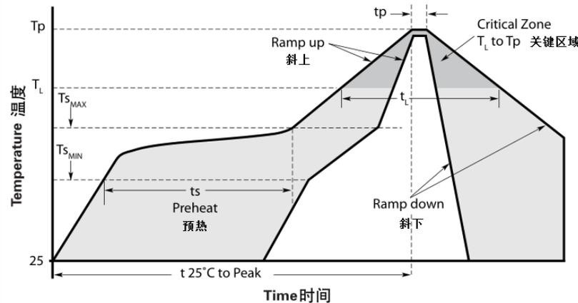
Recommended reflow methods: IR, hot air oven, N2 environment for lead-free. 推荐回流焊方法: 红外线, 热空气, 氮气, 无铅。
