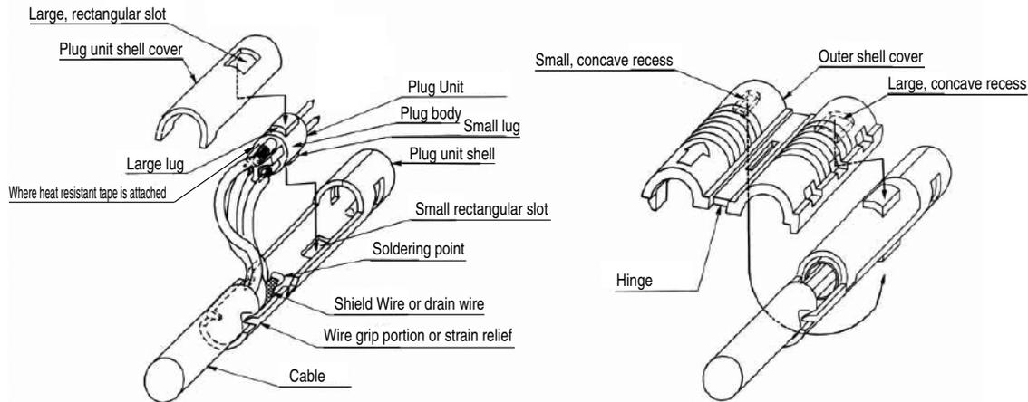
1. Solder the prepared wires of the cable to the plug unit.
