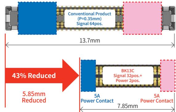
Power lines typically diverted to multiple signal contacts are concentrated into 2 power contacts (Up to 5A/line)
