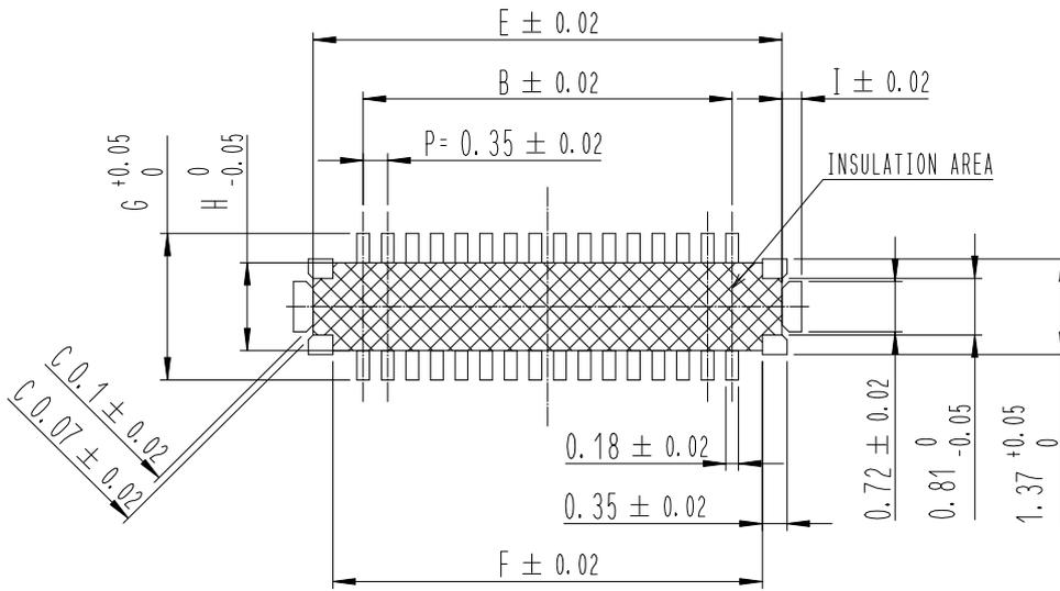
◆ Recommended Metal Mask Dimensions (Mask Thickness : 0.08mm)
