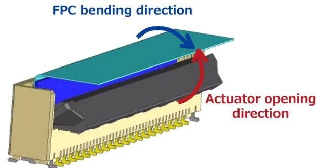
Actuator does not open by bending FPC because actuator opening direction is opposite from FPC bending direction.
