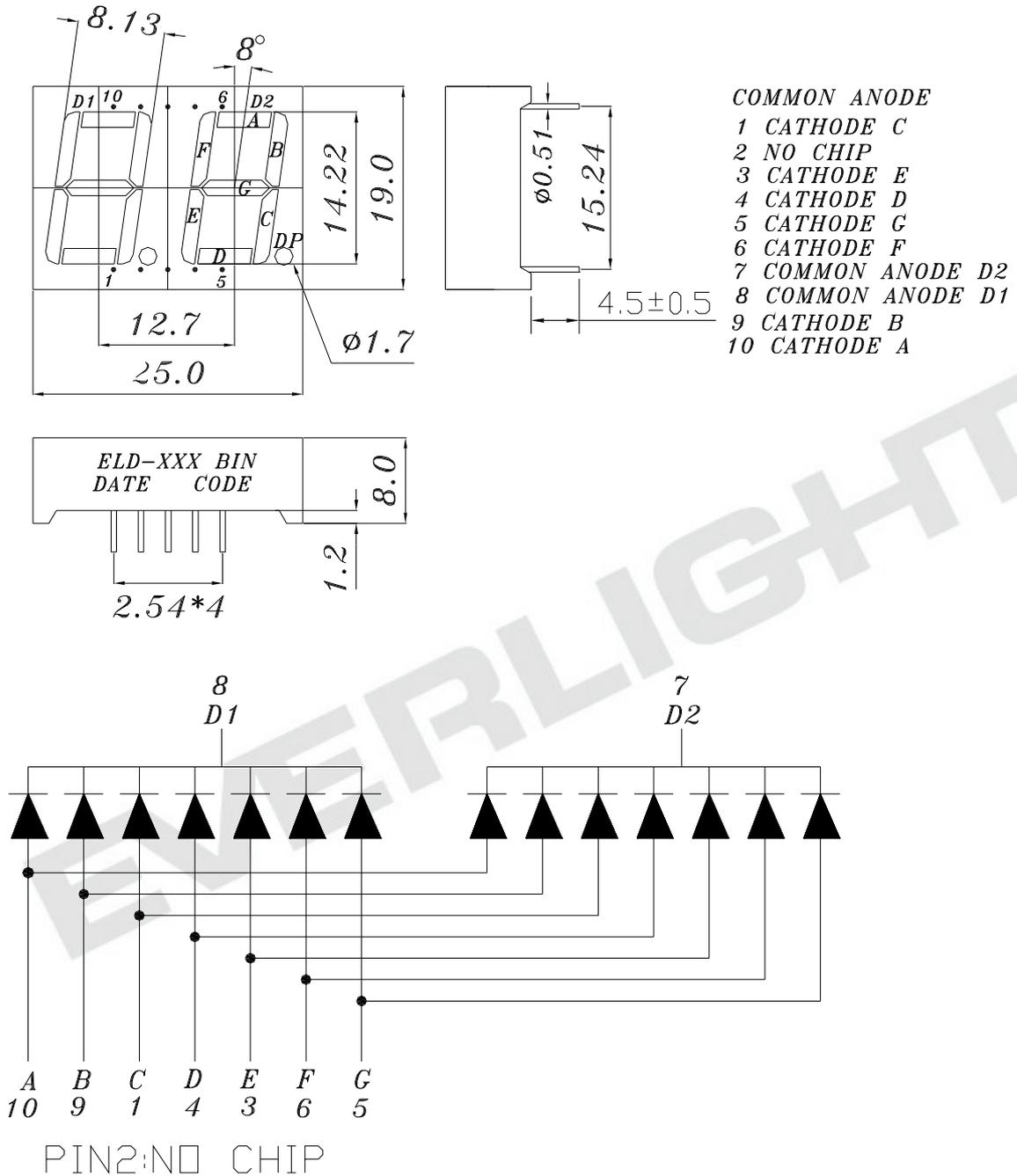
Note: Tolerances unless mentioned ±0.25mm. Unit = mm
