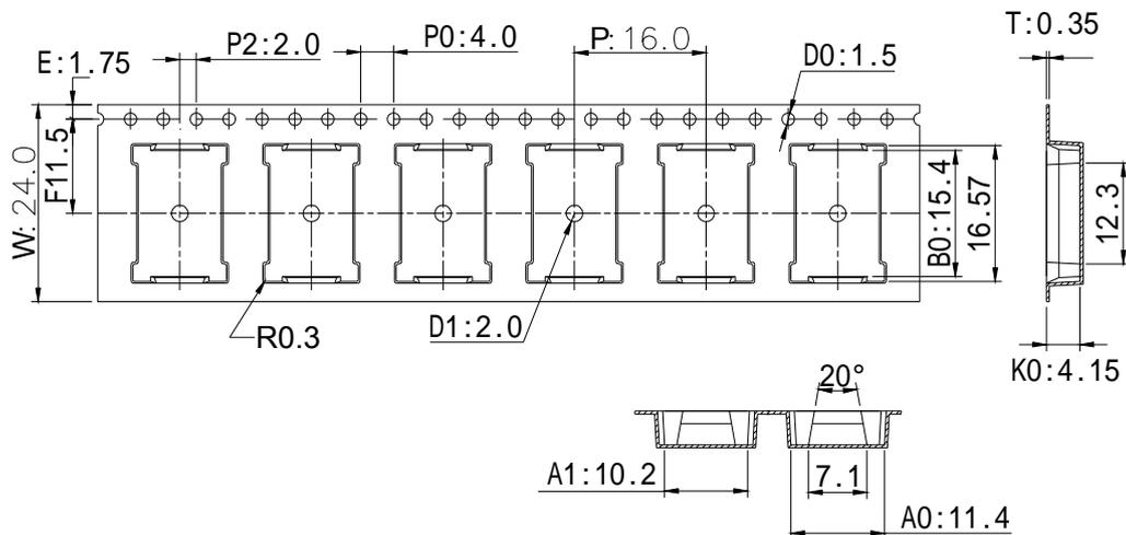
Note: Tolerances unless mentioned  $\pm 0.25\text{mm}$ . Unit = mm
