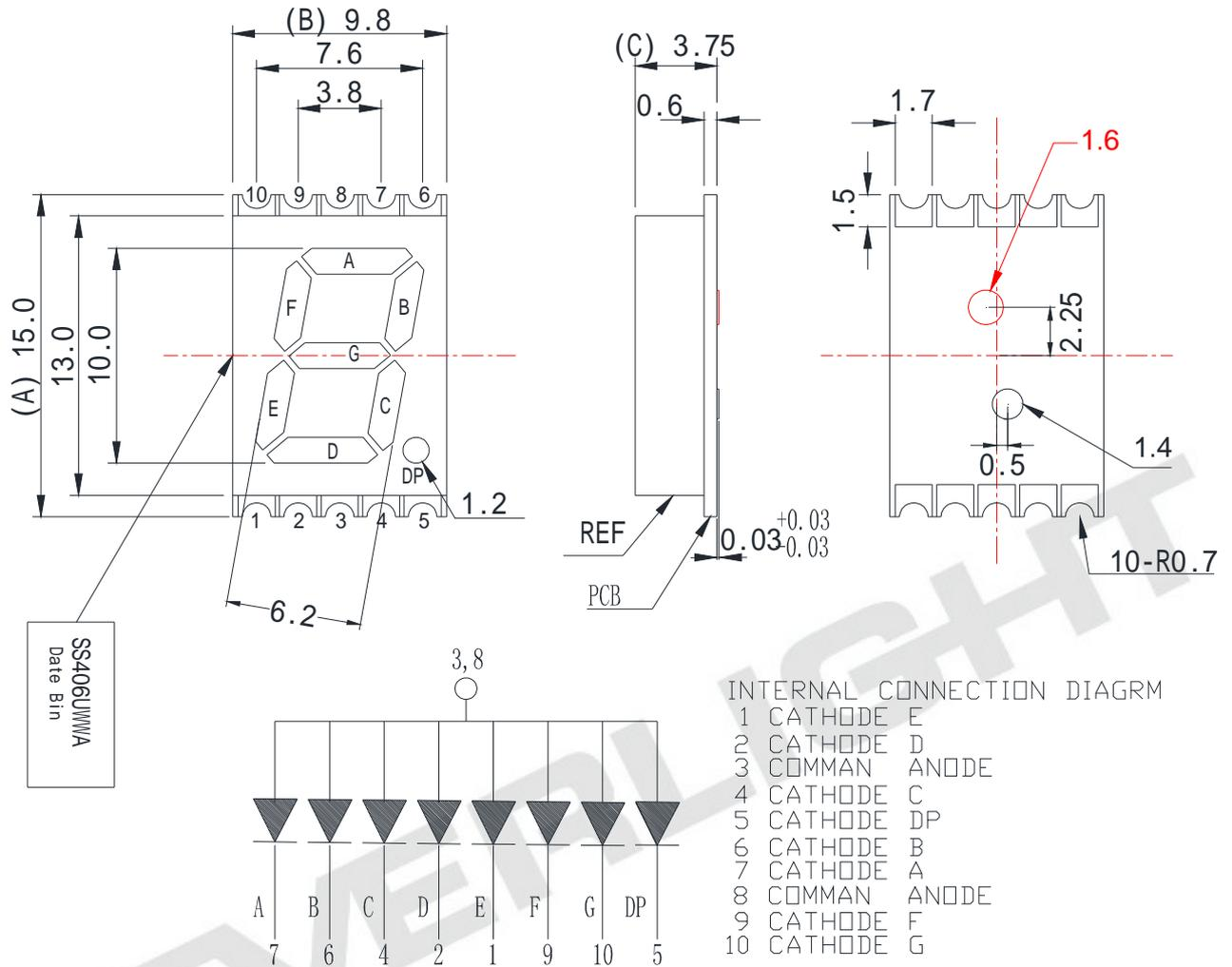
Note: Tolerances unless mentioned  $\pm 0.25\text{mm}$ . Unit = mm
