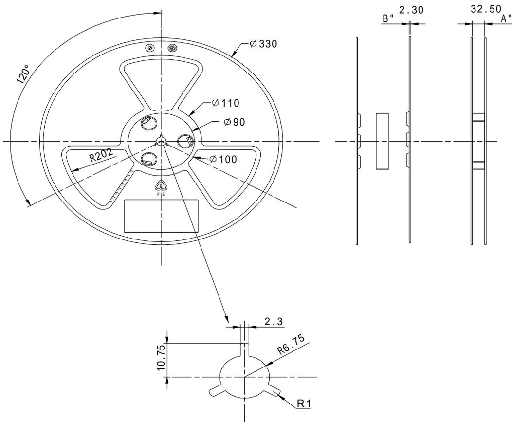
**Carrier Tape Dimensions: Loaded Quantity 800 PCS Per Reel**
