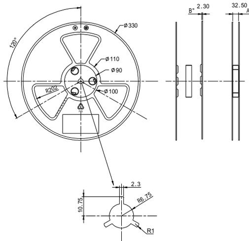
**Carrier Tape Dimensions: Loaded Quantity 800 PCS Per Reel**
