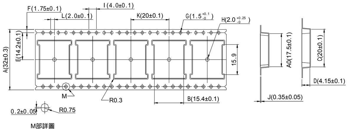
Note: Tolerances unless mentioned  $\pm 0.25$ mm. Unit = mm
