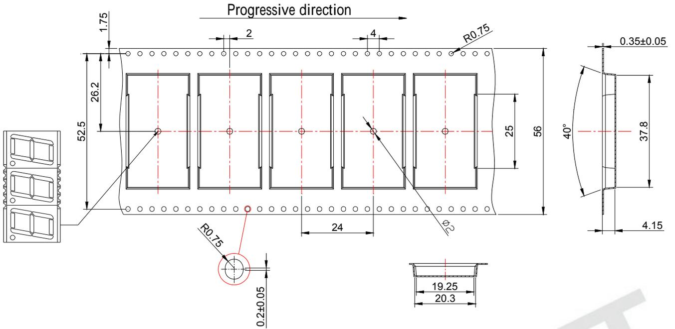
Note: Tolerances unless mentioned  $\pm 0.25\text{mm}$ . Unit = mm
