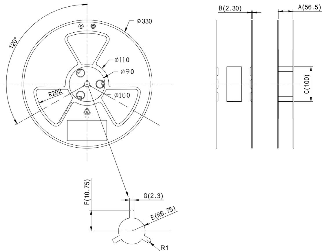
**Carrier Tape Dimensions: Loaded Quantity 500 PCS Per Reel**
