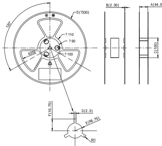
**Carrier Tape Dimensions: Loaded Quantity 700 PCS Per Reel**
