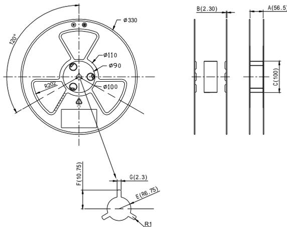
**Carrier Tape Dimensions: Loaded Quantity 750 PCS Per Reel**
