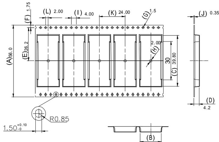
Note: Tolerances unless mentioned  $\pm 0.25\text{mm}$ . Unit = mm
