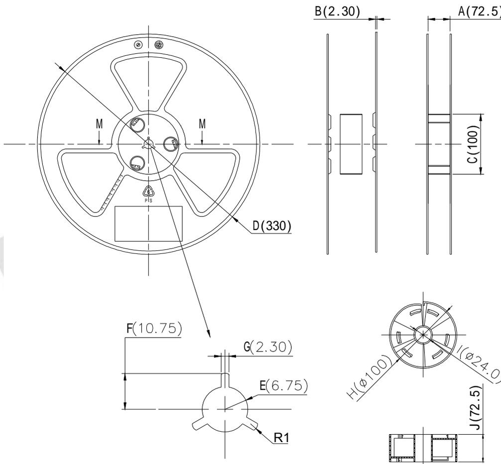
**Carrier Tape Dimensions: Loaded Quantity 600 PCS Per Reel**
