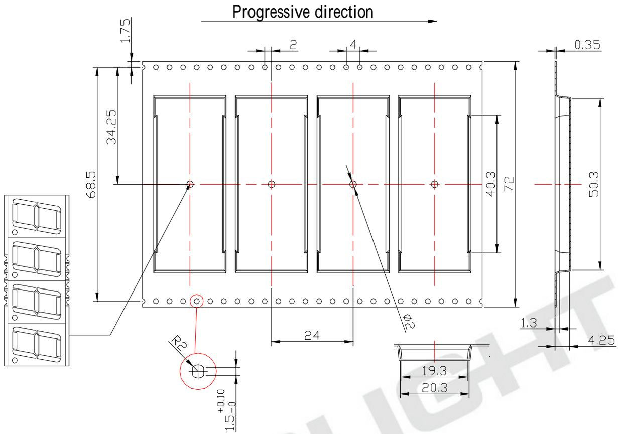
Note: Tolerances unless mentioned  $\pm 0.25\text{mm}$ . Unit = mm
