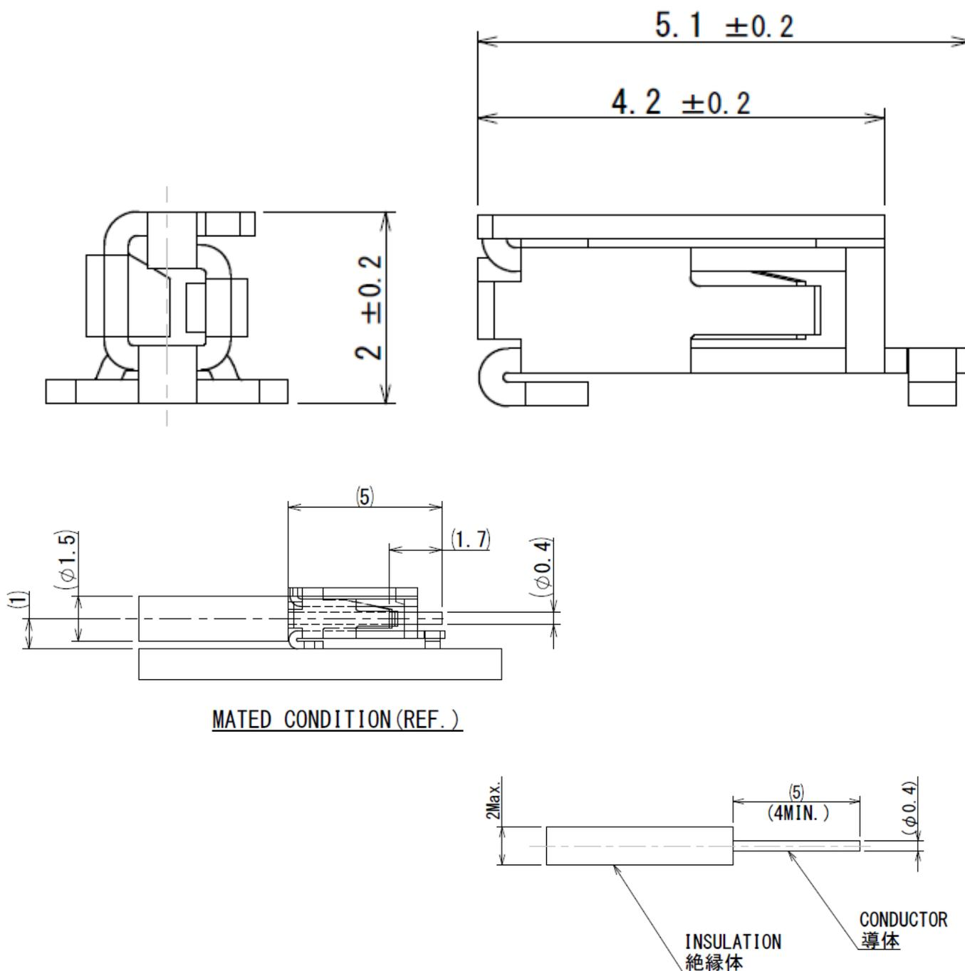
Note 1: Applicable cable (conductor): single wire 26AWG (0.4 Dia.)
