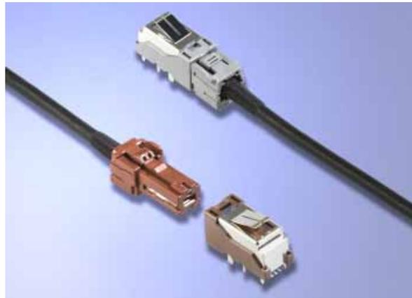
The MX79A Series are miniaturized high-speed automotive infotainment connectors designed to support data transmission. Speeds of up to 1.5 Gbps can be supported when used in conjunction with the MX55J Series of automotive camera connectors. Four mating key variations are available to prevent incorrect mating when multiple connections are used for the same module.
