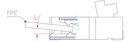
C. FPC Correct insertion verification A visual comparison of the edge of the housing opening and the FPC pattern boundary will prevent diagonal inser-tion and partial insertion errors.
