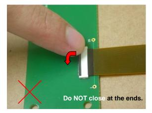
Make surface between actuator and housing be horizontal, it's correct lock position.
