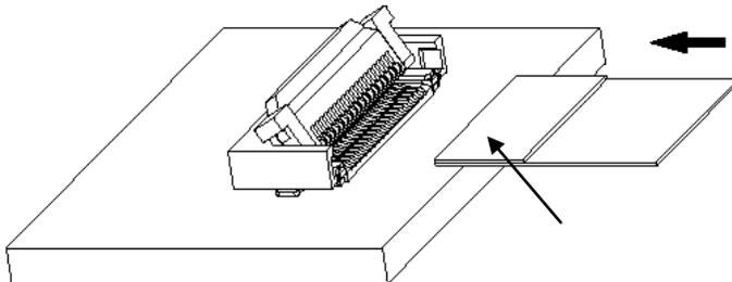
3) Rotate down the actuator until firmly closed. It is critical that the inserted FPC is not moved and remains fully inserted.
