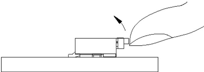
2) Fully insert the FPC in the connector parallel to mounting surface, with the exposed conductive traces facing down.
