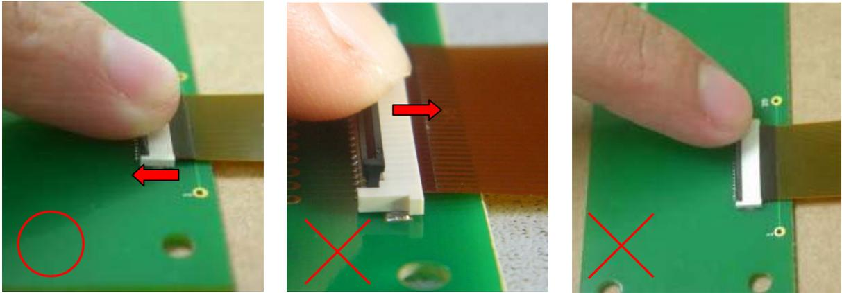
About the lock operation When you lock, it is recommended what the actuator does as a whole, and the actuator was shut surely.
